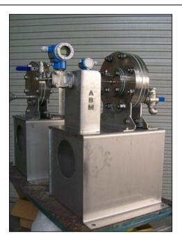
Measuring the Biogas pressure from a Covered Anaerobic Lagoon (CAL) can be unreliable due to the low pressures, typically 0 to 50 Pa (0 to 5mmwg). Wind velocity and ambient temperature can affect the reading combined with the usable span being a fraction of the pressure transmitter's range.
